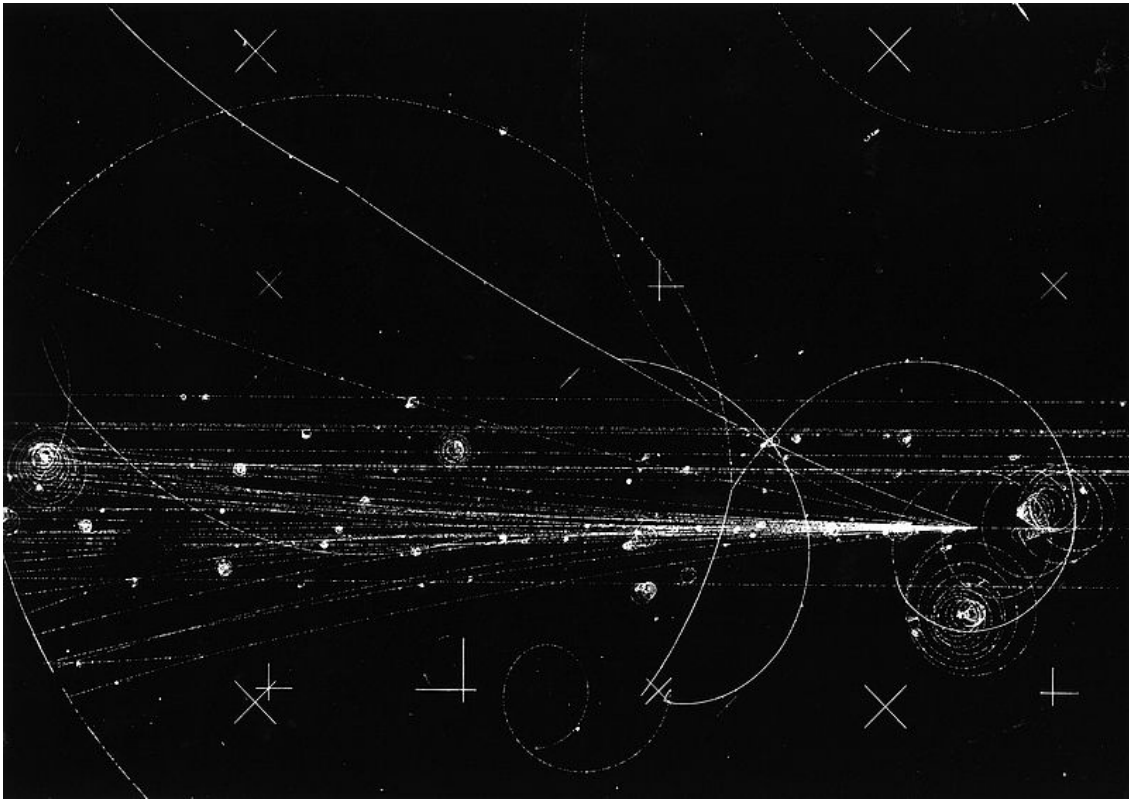
Proton with 300 GeV energy producing 26 charged particles in the 30 inch hydrogen bubble chamber at Fermilab. Source: Wikimedia Commons
